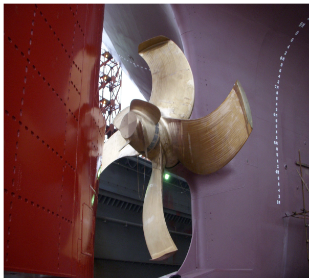
Figure 10. A CLT propeller installed on a bulker, in combination with PBCF and twisted rudder.
