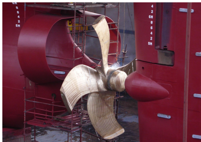
Figure 6. 35,000 DWT product tanker “Roy Maersk”, the new CLT propeller with pre-existing WED and bulbous rudder.
