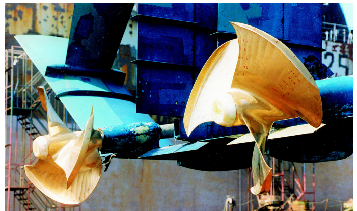
Figure 3. FP CLT propellers installed on an hydrofoil.
