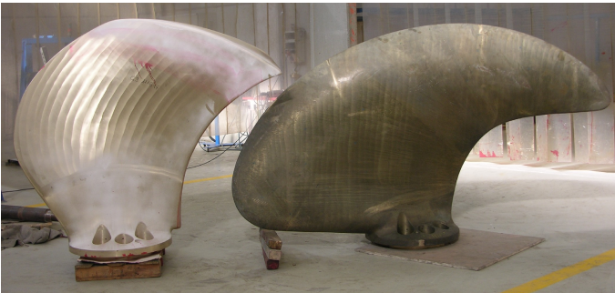
Figure 1. The striking difference between a CLT and a state-of-the-art high skew conventional propeller blade for the same vessel
