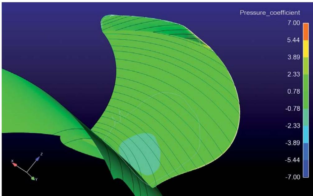
experimental results (up to 6.5% error on  $KT$  and 16.5% error on  $KQ$ ).
