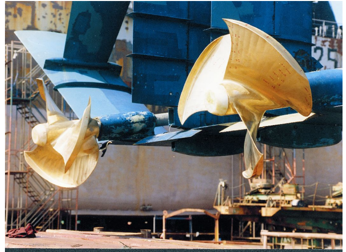
Figure 4. FP CLT propellers installed on an hydrofoil.
