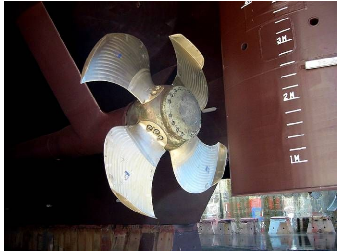
Figure 5. A CP CLT propeller installed in a modern Ro-Pax.
