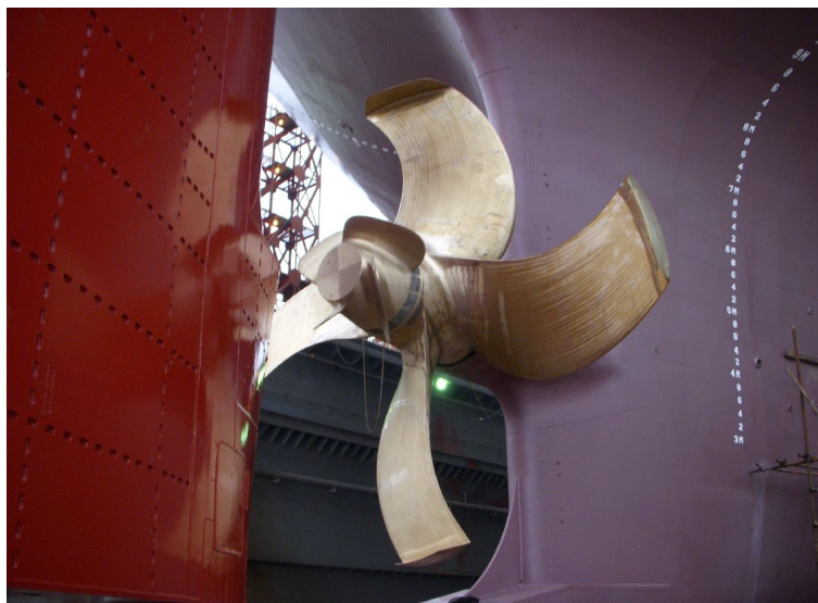
Figure 10. A FP CLT propeller installed on a bulk carrier, note the pre-existing PBCF and twisted rudder
