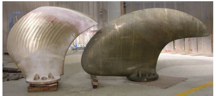
Figure 1. The striking difference between a CLT and a state-of-the-art high skew conventional propeller blade designed for the same Ro-Pax.
