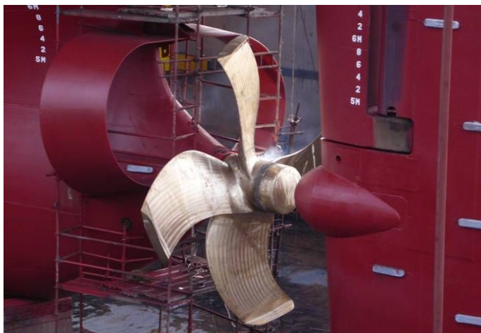
Figure 6. 35,000 DWT product tanker “Roy Maersk”, new CLT propeller and pre-existing WED.
