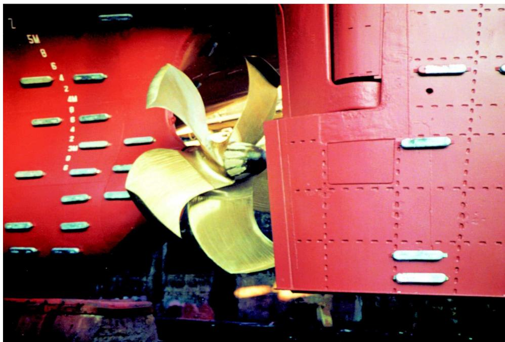
Figure 1. A 5 bladed FP CLT propeller installed on a containership.
